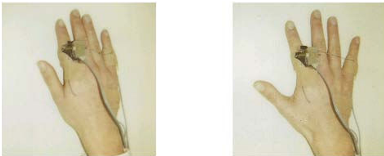
Figure 1 Device to register reactions. Device to register reactions (spreading of the hand with the m. abductor digiti minimi involved). left side: switch open, right side: switch closed.
